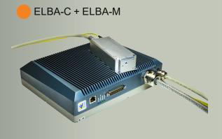
Output power up to 3 W 520, 532, 546, 560 and 577 standard wavelengths, ...
